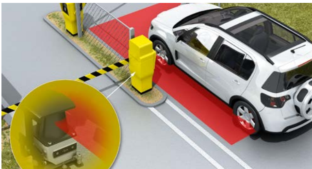
Barrier control with the TiM351 as an induction loop replacement.
